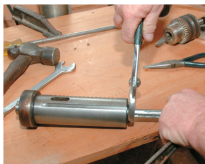
Tightening the bearing nut to pre-tension the bearings
