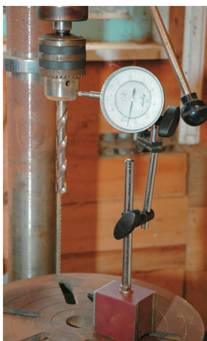
Measuring the run-out at the chuck
