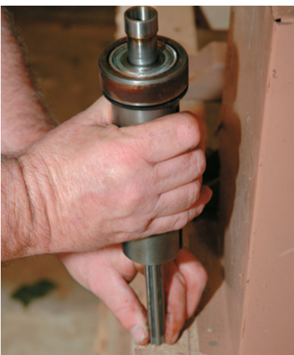
Removing the quill shaft
