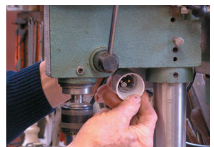
Fix lamp in place.
