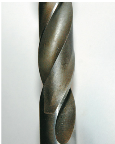
Drill showing the body relief ground into the spirals. This helps to reduce friction.
