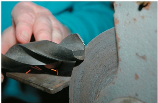
Relieving or grinding away the web, blending the web into the flutes.
