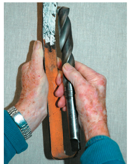
Morse taper drill gauge. The lines scratched on the chalked area by the cutting wings should match. Note spike fitting in the end of the drill.
