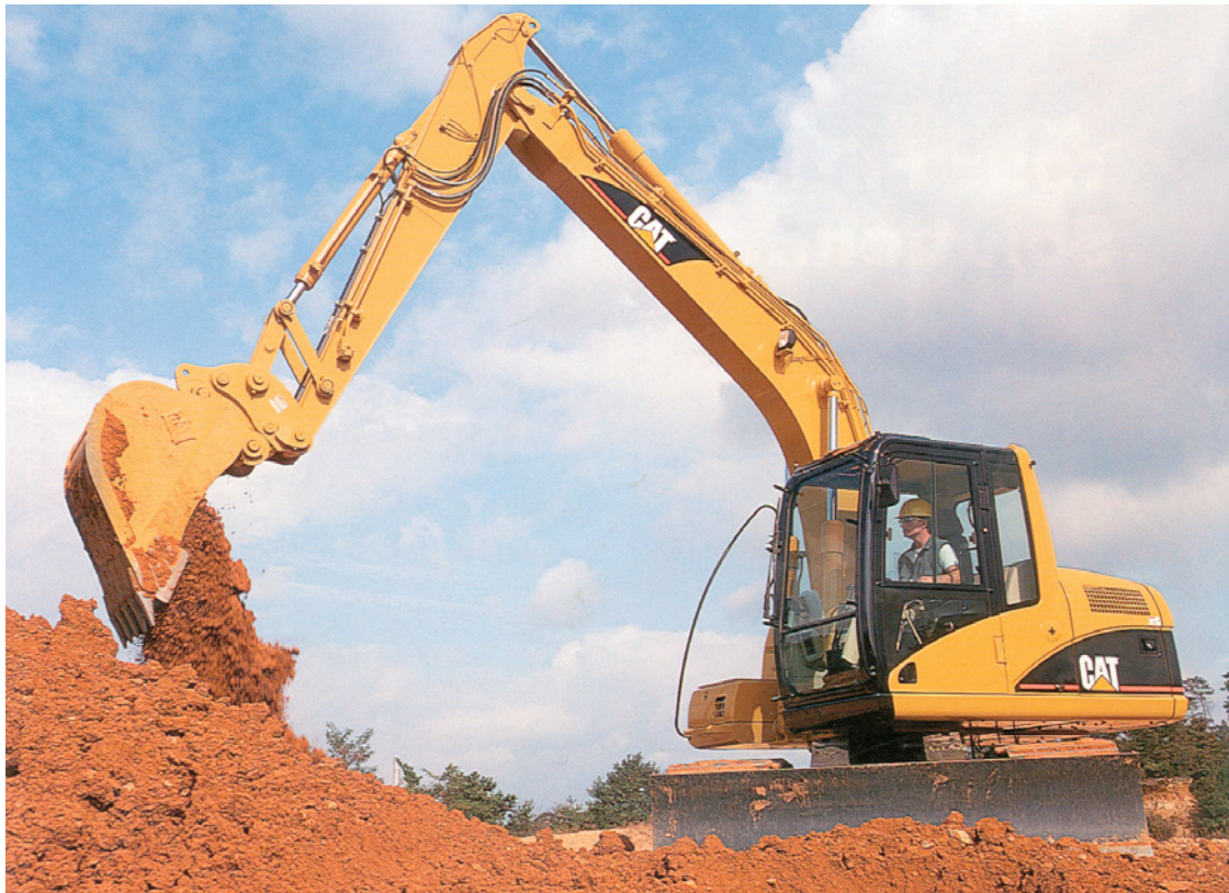
Hydraulics at work: A Caterpillar excavator showing the combination of hydraulic rams which work the bucket.
