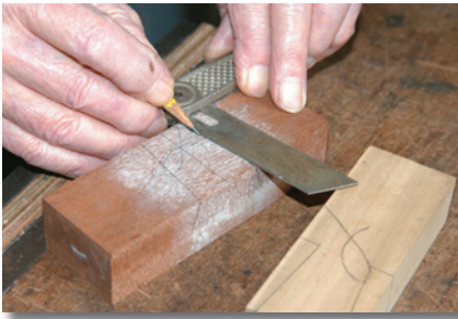
Marking up. Chalk on mahogany socket wood brings out marks.
