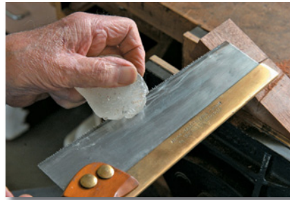
Wax lubricates tenon saw.
