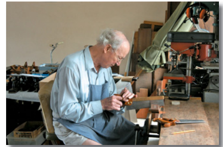
Tenon saw in action. Note wood at angle so cut is vertical.
