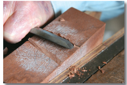
Remove waste with chisel.
