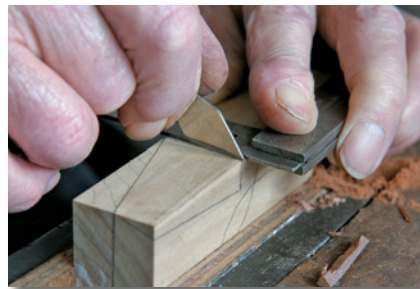
Cut pin shoulders with sharp knife.
