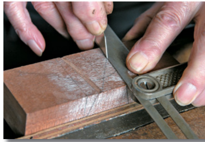
Cut slope with sharp knife.
