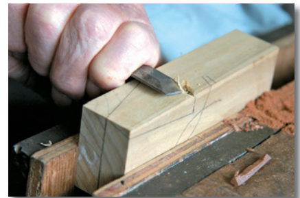
Chisel forms ledge to guide saw.
