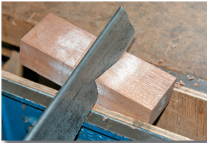
Fine-toothed saw cuts compound angles.
